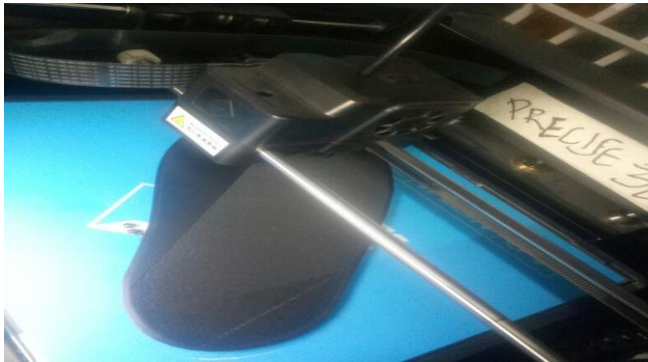
Fig-6.2.2: Formation of Second Layer
