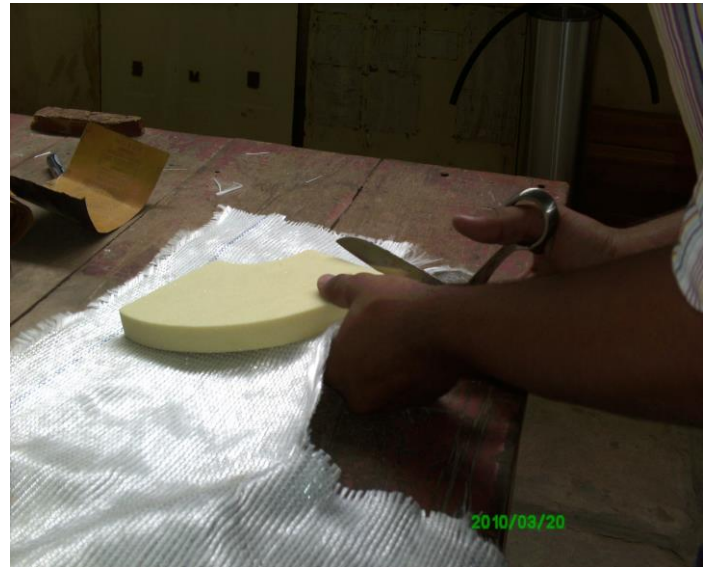
Fig 3.6: The woven fabric cloth is cut into the required shape of the mould and laid inside the mould
