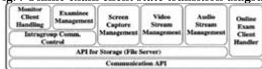
Fig. . Monitor server architecture.
