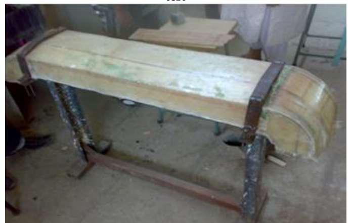
Fig 3.11:FRP Sandwich bumper fixed to Rigid Metallic frame to conduct the deflection test
