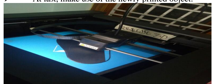
Fig-6.2.1: Formation of First Layer in 3D Printing
