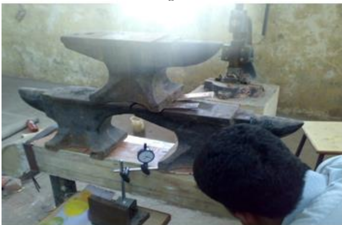
Fig 3.13: FRP Sandwich bumper deflection test inprogress 150Kg
