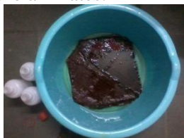
Fig.3. Pretreatment (Alkali Noah) of the fibers and the jute material
