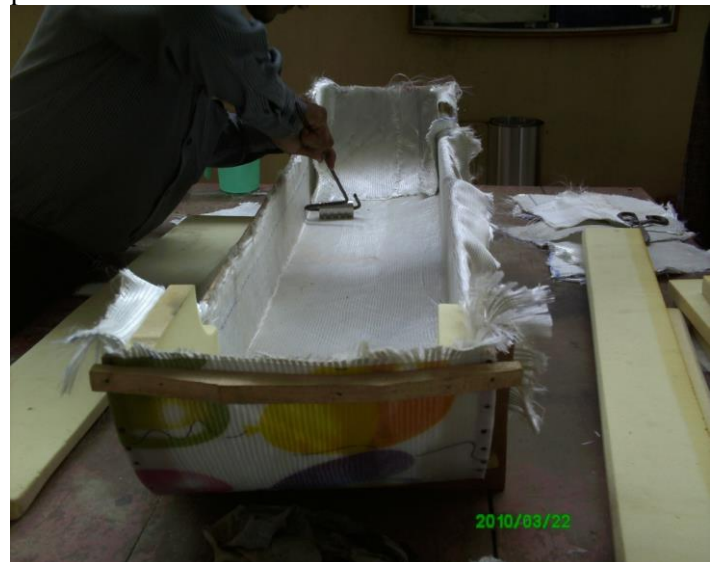
Fig 3.7: Applying a resin lay up
