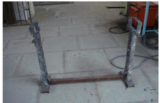
Fig 3.10: Rigid Metallic frame to conduct the deflection test
