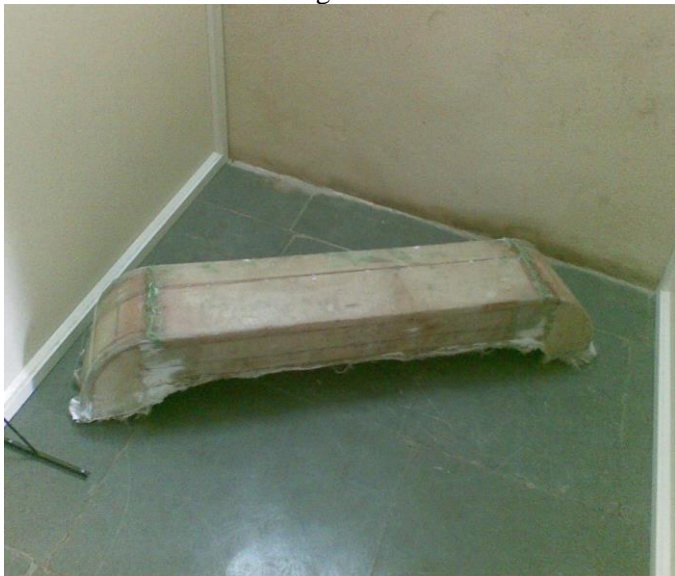
Fig 3.9: After the removing the wooden mould
